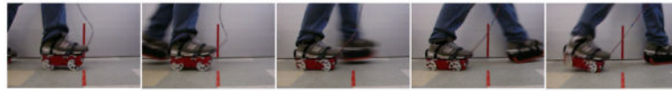
Fig. 6. GEMS from heel contact until toe off. The GEMS was measured to have a smooth horizontal backward motion of 6" (15.2 cm). Note that one floor tile is 12" (30.5 cm). These images are taken from the included video.
