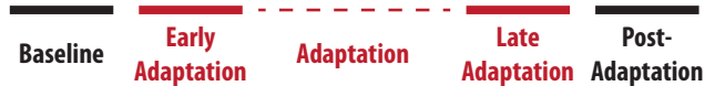
Figure 6. Experimental paradigm. Solid lines show periods that were recorded. The dashed line (adaptation) was not recorded. Subjects wore the GEMS during the red periods, and walked in normal sneakers for the black periods (Baseline and Post-Adaptation). All of the recorded periods consisted of ten trials. A trial was equivalent to 1 pass across the over ground walking path, which took 8-12 steps. The unrecorded adaptation period (dashed line) lasted 10 min, which was equivalent to 309.3 \pm 56.5 steps (mean \pm SD).
